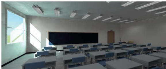
A Radiance simulation shows the penetration of daylight into the interior of the classroom at 3pm in March with only vision glass for glazing.
