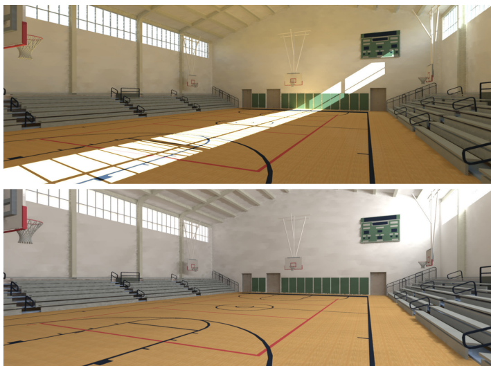
Daylight models with vision glass (top) and Solera engineered daylight diffusers (bottom).
